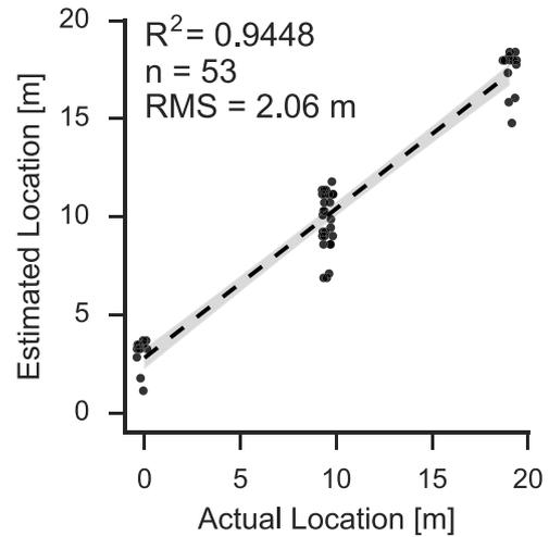
Fig. 4. Linear regression between known tag locations and locations estimated with the TDOA system, shaded area is the 95% confidence interval.
