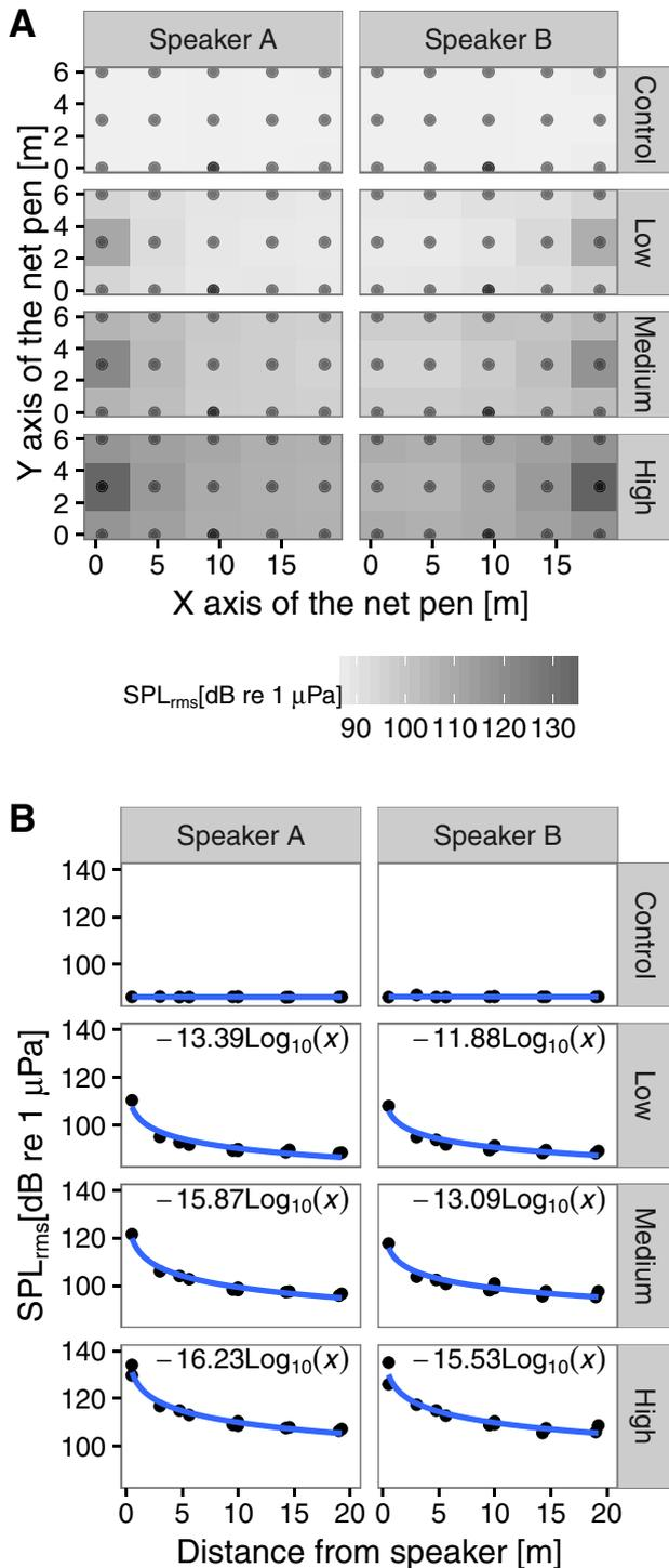
**Fig. 1.** (A) SPL<sub>rms</sub> measured within the experimental pen at each volume level; points indicate locations where the SUR measured SPL<sub>rms</sub>. Location measurements are assumed along the long (x) axis of the pen only. (B) Fitted transmission loss log functions for each volume x speaker combination.
