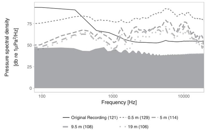
**Fig. 2.** Pressure spectral densities calculated from recordings at the high volume level taken at four distances from the underwater speaker compared to the original recording of the ORPC hydrokinetic turbine and ambient conditions in the quarry. Corresponding SPL<sub>rms</sub> values for each recording are included parenthetically in the legend. Filled area indicates ambient pressure spectral density and assumed consistent across test conditions.
