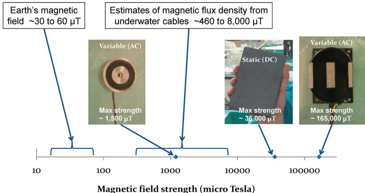
FIGURE 1. Maximum field strengths ( $\mu\text{T}$ ) measured at the surface of the AC and DC magnets used in this study, presented in comparison with the Earth's natural field strengths and with field strengths predicted for underwater transmission cables. [Figure available online in color.]
