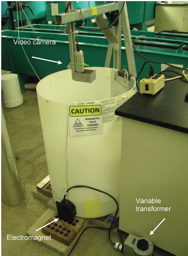
FIGURE 4. Experimental tank used to test the responses of juvenile Paddlefish and Lake Sturgeon to a 4-s burst of electromagnetic field created by an AC electromagnet. [Figure available online in color.]
