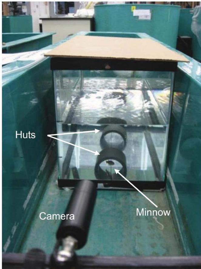
FIGURE 2. Experimental setup for the 46-h electromagnetic field exposure experiments. [Figure available online in color.]
