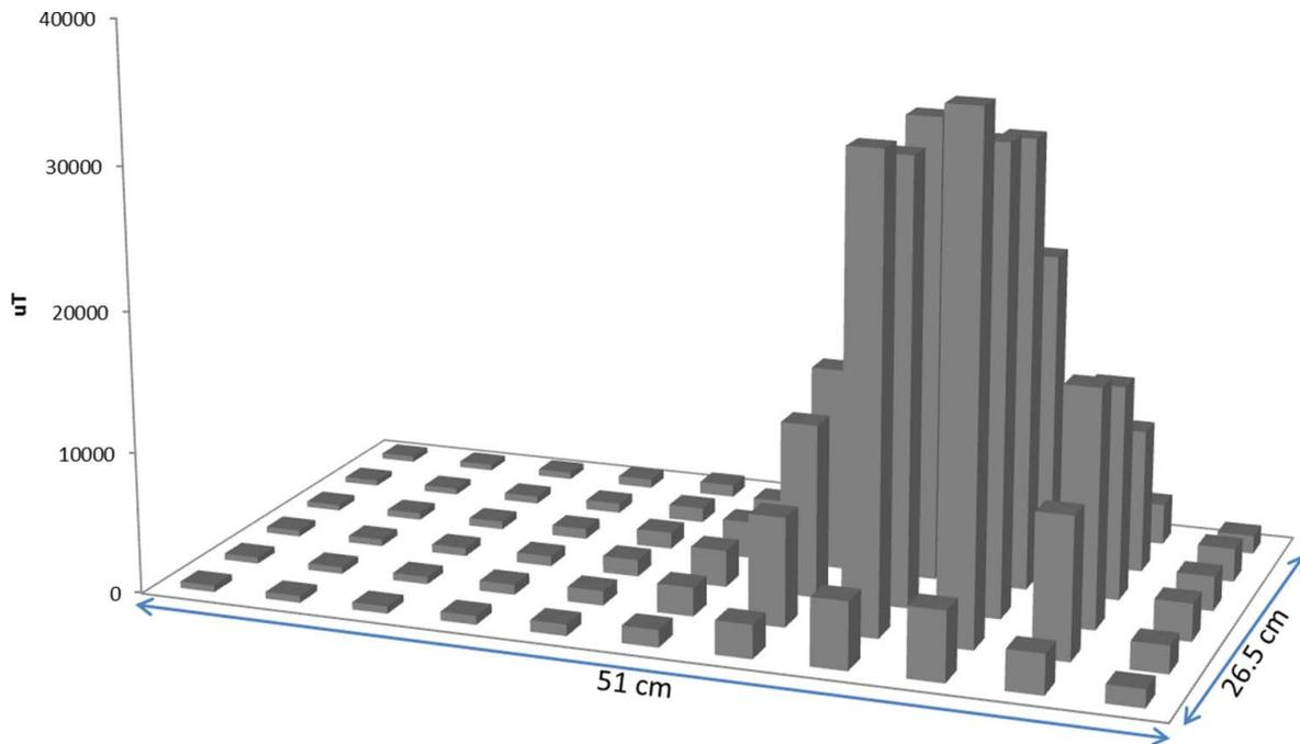
FIGURE 3. Strength ( $\mu\text{T}$ ) of the static magnetic field created within each aquarium when placed over a permanent bar magnet. The maximum field strength was 36,410  $\mu\text{T}$ . [Figure available online in color.]
