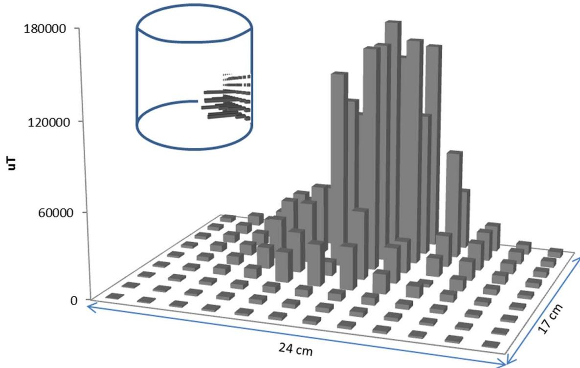
FIGURE 5. Magnetic field ( $\mu\text{T}$ ) produced at the inside wall of an experimental tank (i.e., as depicted in Figure 4) by an AC electromagnet at the strongest (100%) setting. The far row represents the bottom of the inside of the tank, and the embedded schematic of the experimental tank shows the placement of the field as the fish would have experienced it. [Figure available online in color.]
