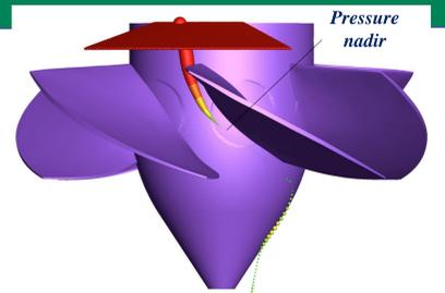
Schematic of a turbine runner that depicts the drop in water pressures to low values (nadirs) that are injurious to fish.
