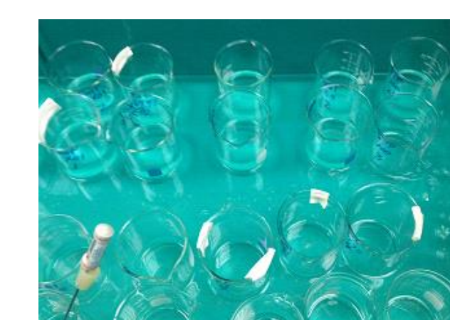
Ceriodaphnia reproduction and survival toxicity test set-up (left); fathead minnow chronic larval growth and survival test (right)
